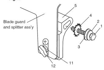
4. Install the blade guard and splitter assembly (6) into the rear of the saw table. Thread the bolt (1-Fig. H) into the internally threaded pivot rod (7) until snug.
